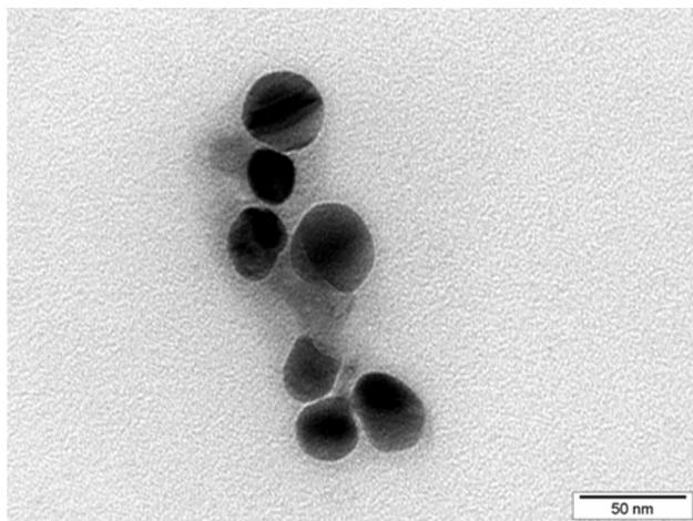
Fig. 2. TEM micrograph of the synthesized Ag nanoparticles.
