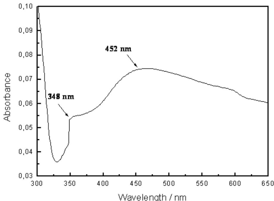
Fig. 4. UV-visible spectrum of the synthesized silver nanoparticles.
