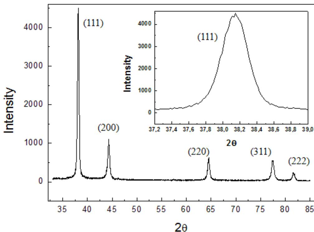
Fig. 3. XRD patterns of the synthesized Ag powder. Inset: The broadening of the intense (111) diffraction peak.
