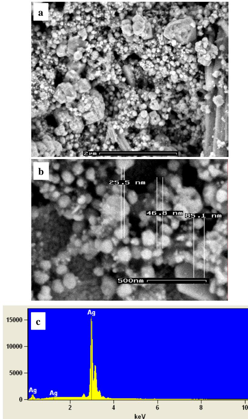
Fig. 1 a) and b) SEM micrographs of the synthesized Ag nanoparticles with different magnifications. c) EDX profile of Ag nanoparticles.
